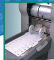
Automatic extending conveyor activated by the number of forms processed
